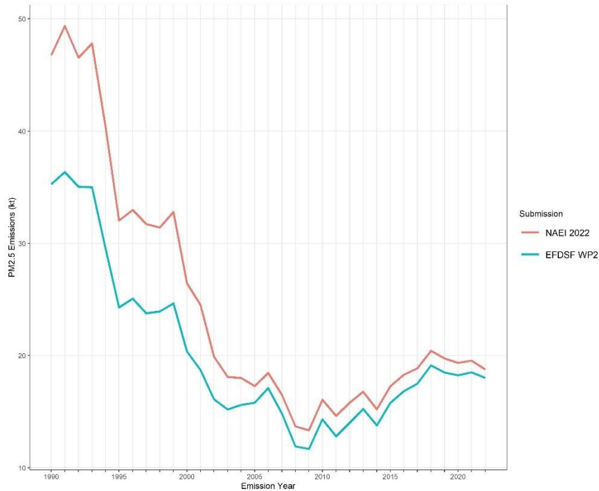
Figure 6-25 Historic impact of new EFs on PM 2.5 emissions in domestic combustion sector
