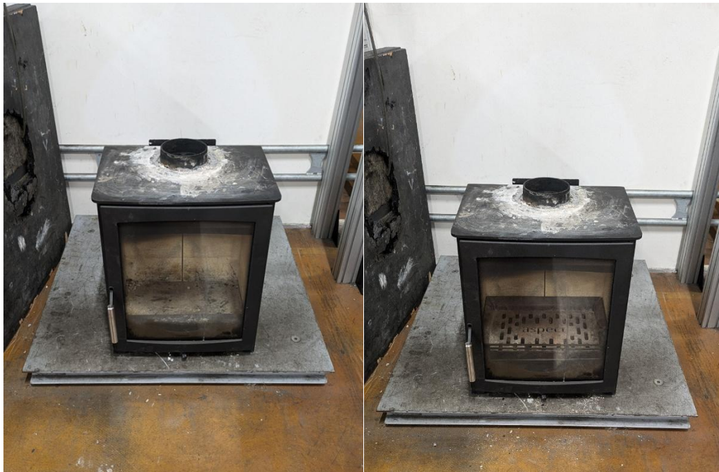
Figure A-2- 7 - Images of the Hunter Aspect 5 in wood only configuration (left) and multifuel configuration (right)
