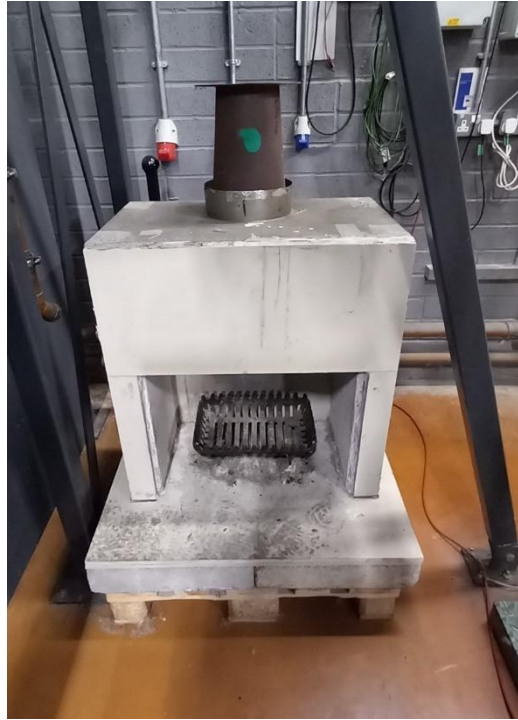
Figure A-2- 4 - Images of the Cromwell Fire basket (Open Fire) used in the test programme
