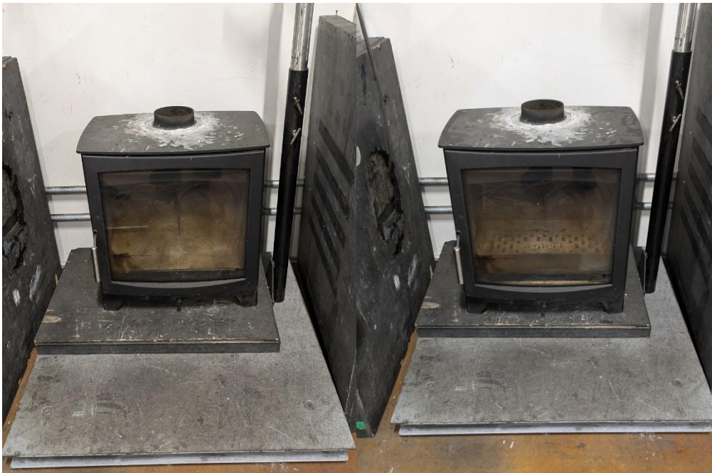
Figure A-2- 9 - Images of the Hunter Aspect 8 in wood only configuration (left) and multifuel configuration (right)
