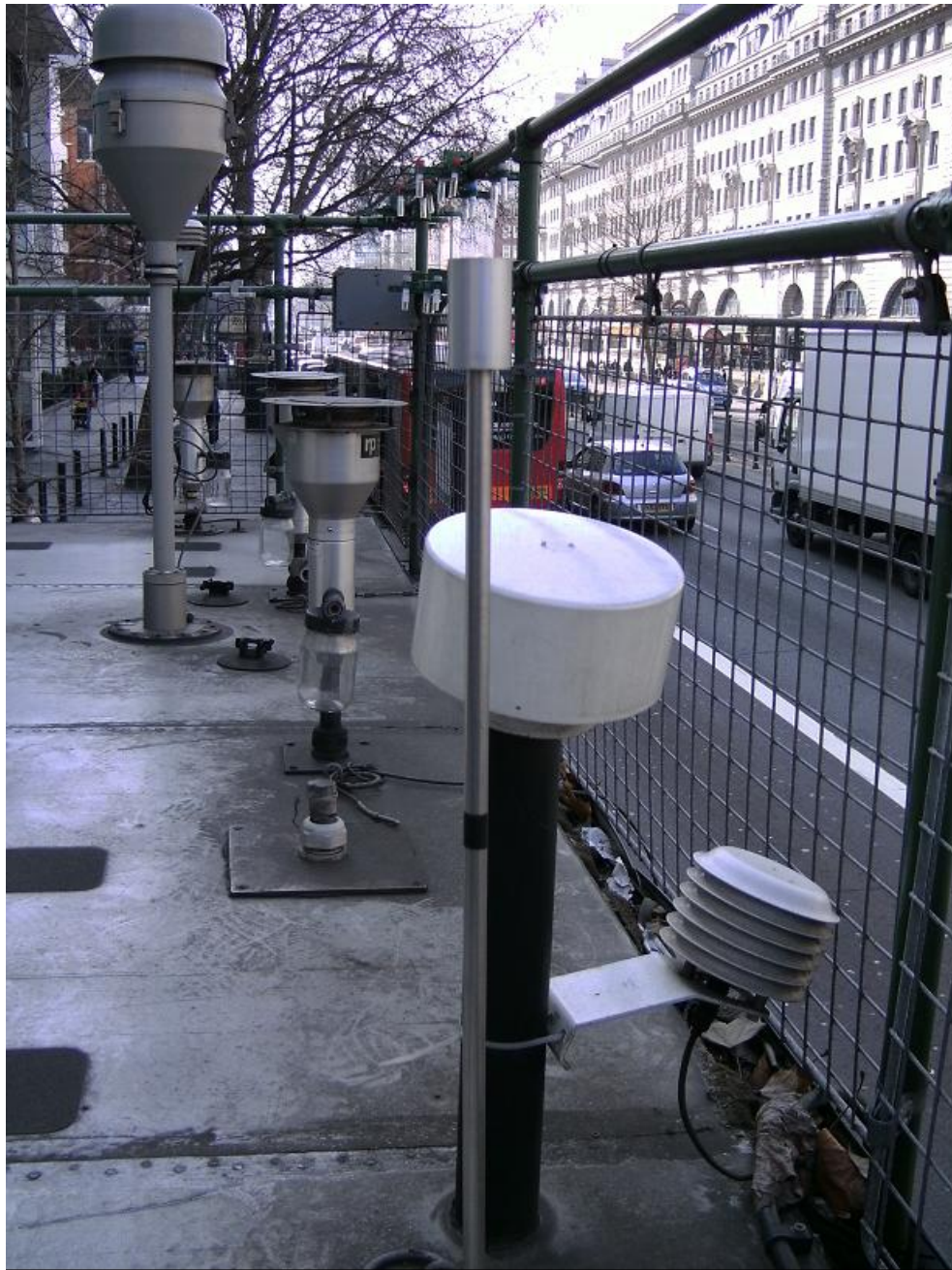
Figure 3b Stainless Steel Rain Cap And Inlet Pipe Work For The Aethalometer At The Marylebone Road Site
