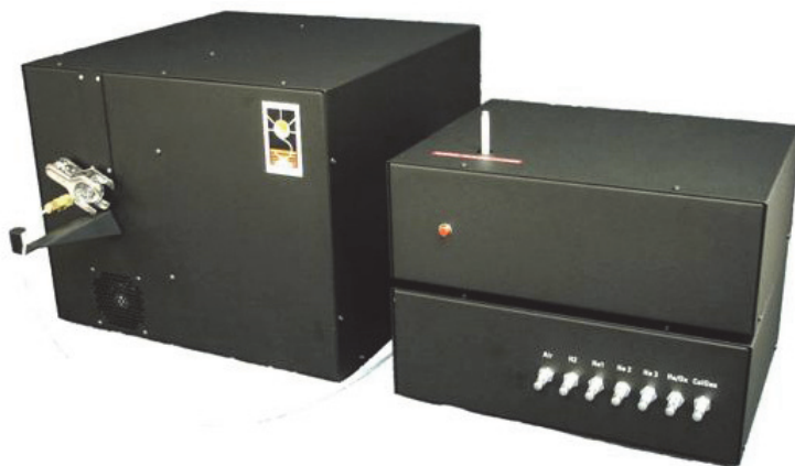
Figure 2-4 Sunset Laboratory Inc. thermal/optical carbon analyser
