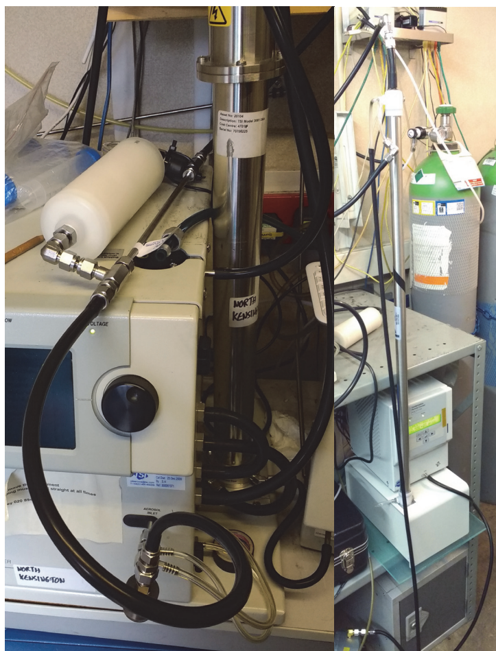
Figure 2-2 Typical configuration of CPC, SMPS and drying units at the Network sites
