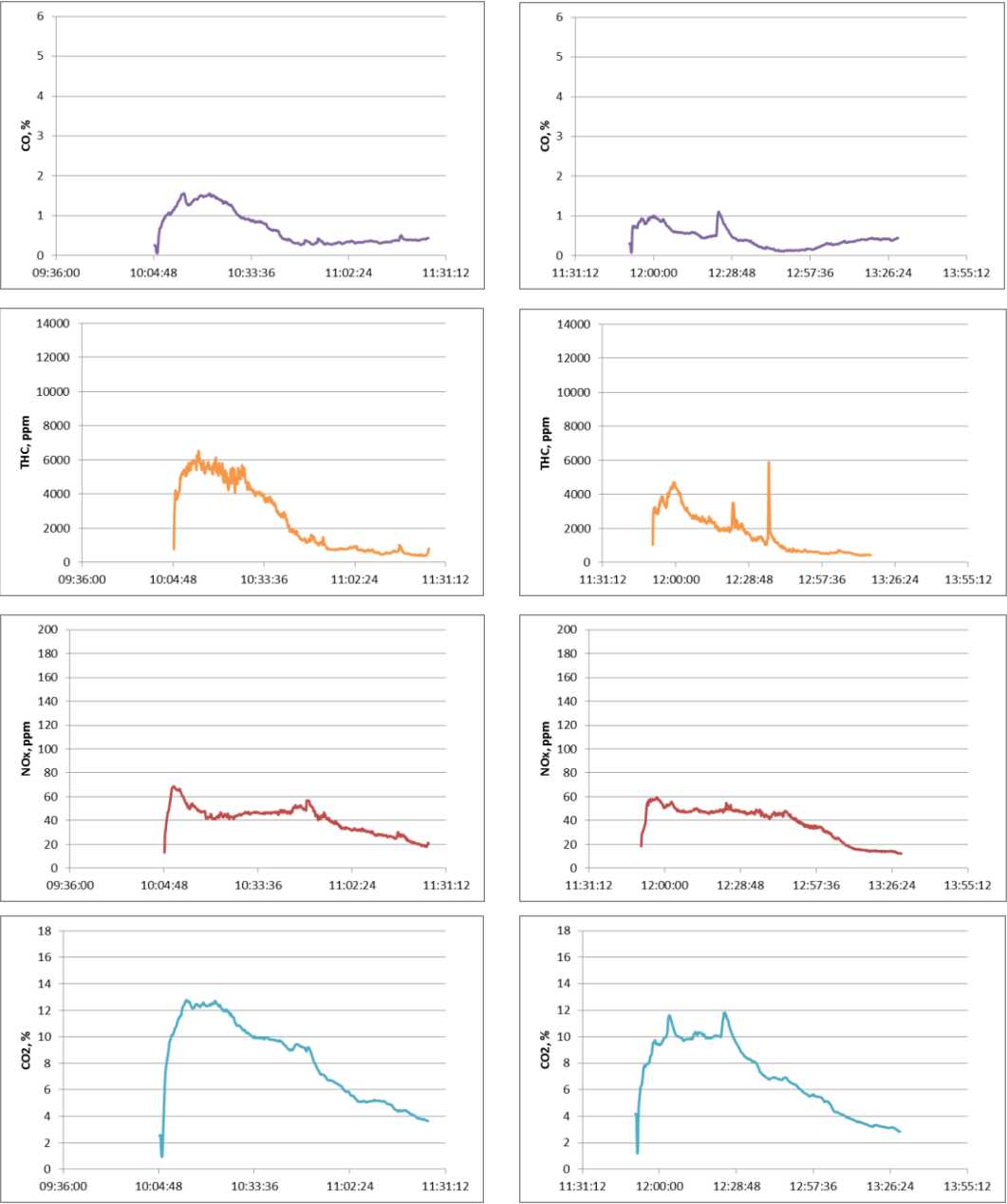
Figure A1.4f Flue gas measurement traces of CO, THC, NOx and CO 2 for Appliance D, DIN+, High Output, Test 1 (left) and Test 2 (right)
