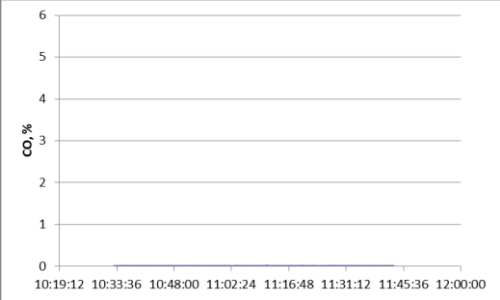
Figure A1.6a Flue gas measurement traces of CO, NOx, THC and CO 2 for Appliance F, ESP, High Output, Test 1 (left) and Test 2 (right)
