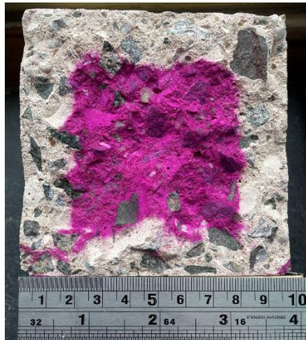
Figure 1 Phenolphthalein indicator test - CEM III/A concrete (31.9MPa 28-day strength) tested at 17 years
