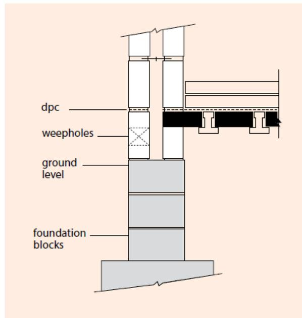
Figure 25 Detail of blockwork foundations for masonry construction<sup>53</sup> (dpc indicates the damp-proof course)
