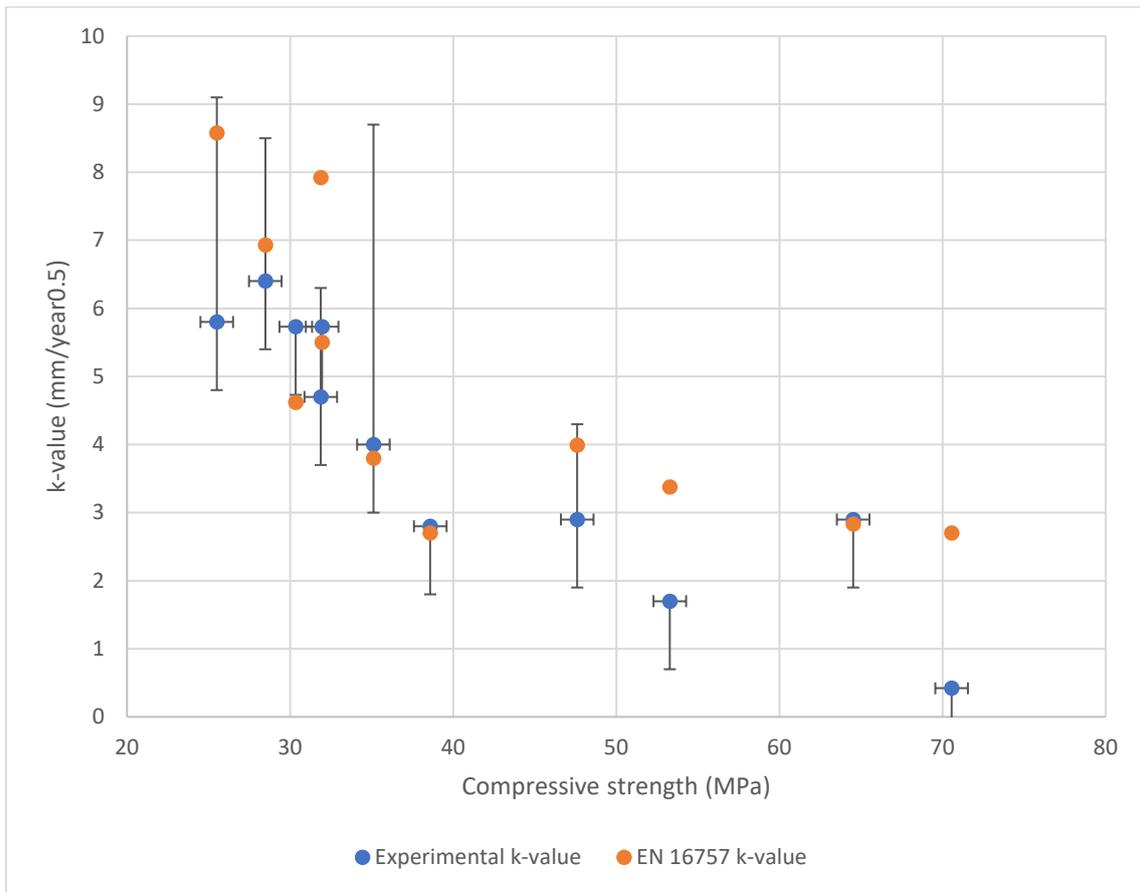
Figure 26 Comparison of experimental k-values with empirical values from EN 16757 for various concrete strengths
