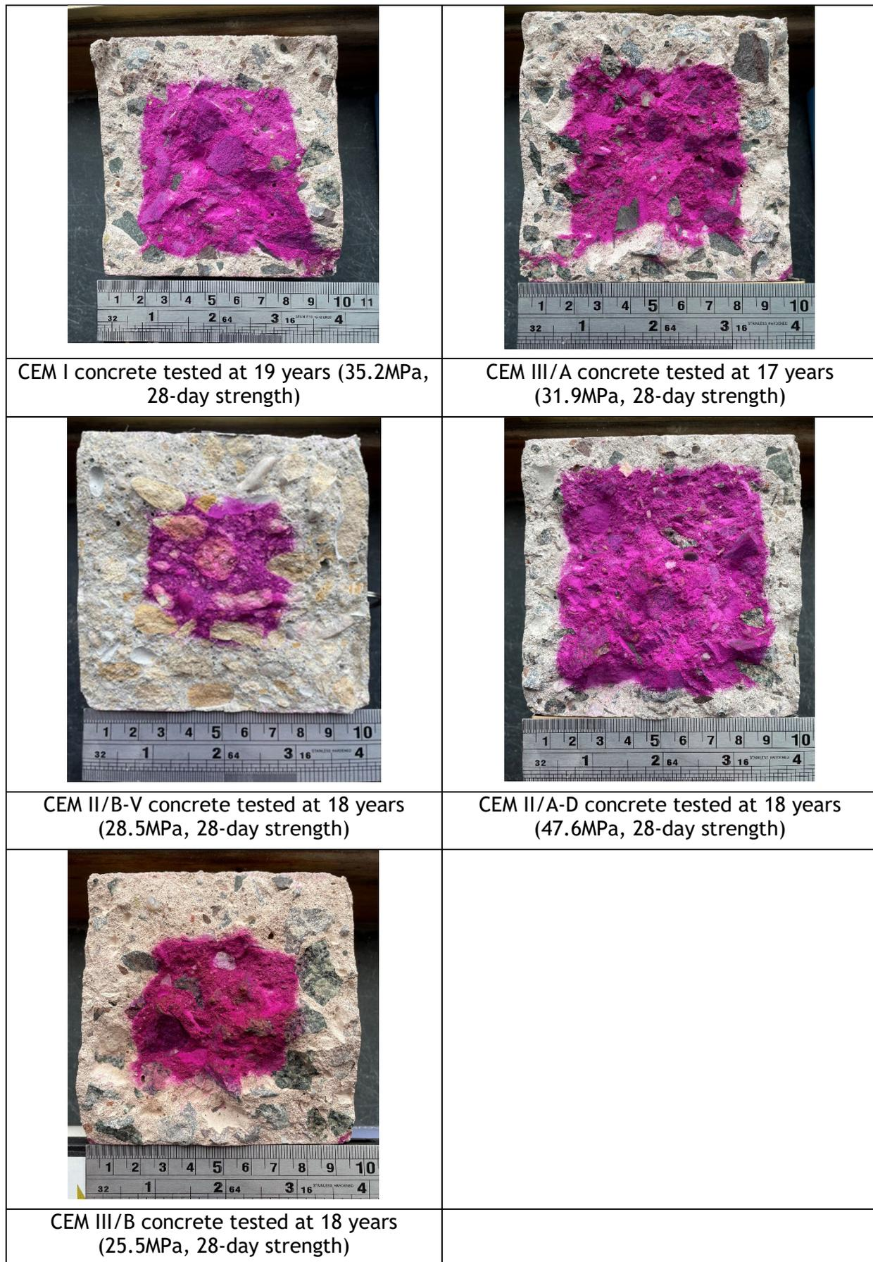
Figure 13 Concrete prisms tested for carbonation depth at the University of Dundee
