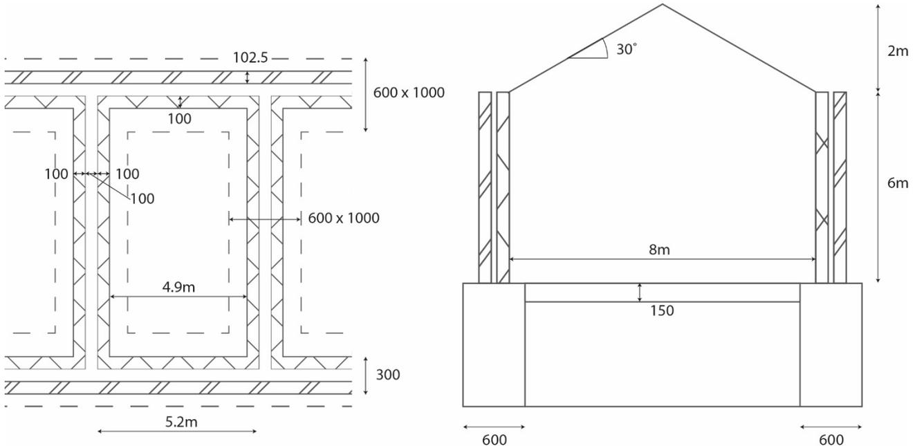
Figure 22 Plan and cross-section of 2-bed, 2-storey mid-terrace masonry house
