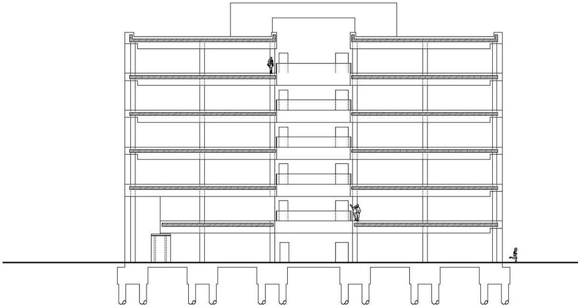
Figure 7 Cross-section of steel composite frame office building
