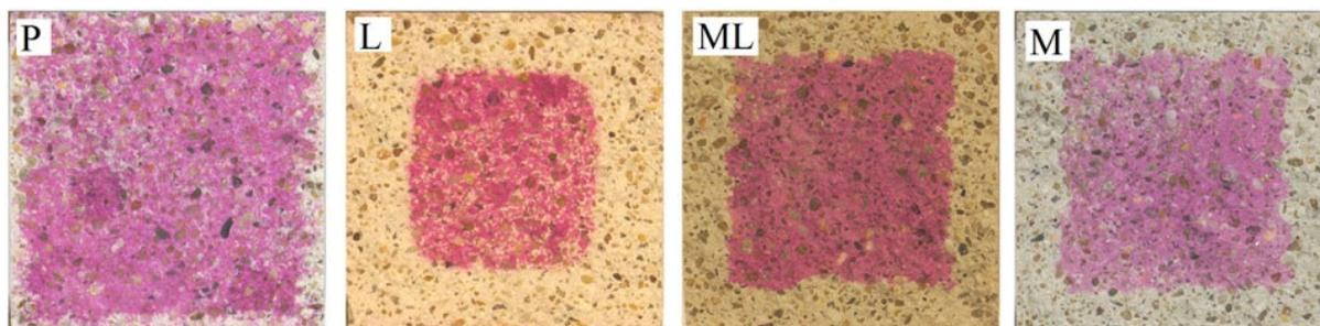
Figure 4: Carbonation depth measured using the phenolphthalein indicator (from Shi et al.,<sup>36</sup>).
