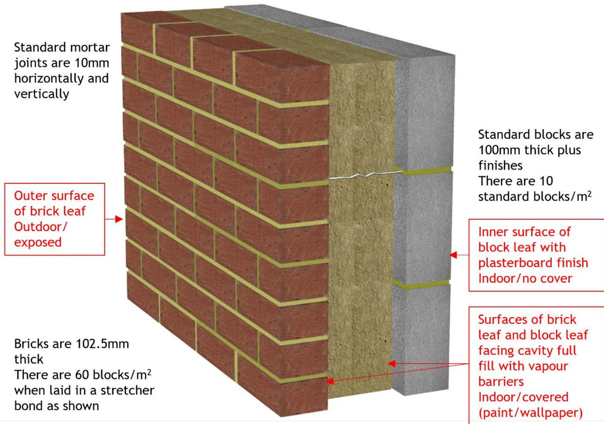
Figure 24 Cavity wall construction for external wall of masonry house. Also used for external walls of concrete-frame residential apartment building. Callout boxes show exposed surfaces used in the EF calculations.
