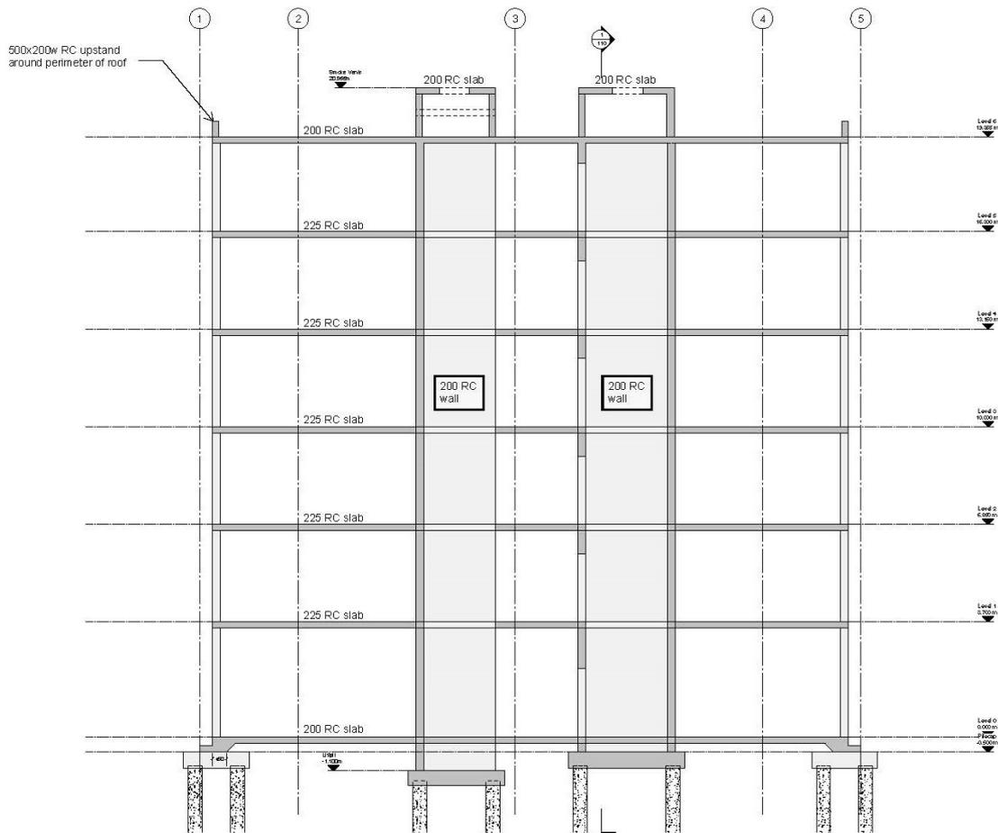
Figure 21 Cross-section of concrete-frame residential apartment block
