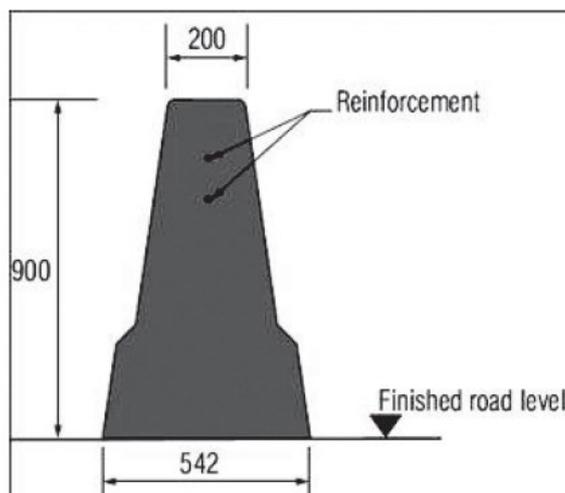
Figure 23 Typical geometry of concrete barrier (Britpave 2008: Barrier Cost Comparison)
