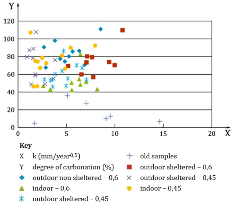
Figure 5: The degree of carbonation (y-axis) against carbonation rate k (x-axis). 0.6 and 0.45 refer to the water-cement ratio used when manufacturing the test samples. ‘Old samples’ refers to material collected from existing structures (in service for 10-20 years prior to sample collection), Source CEN/TR17310<sup>40</sup> and references therein.
