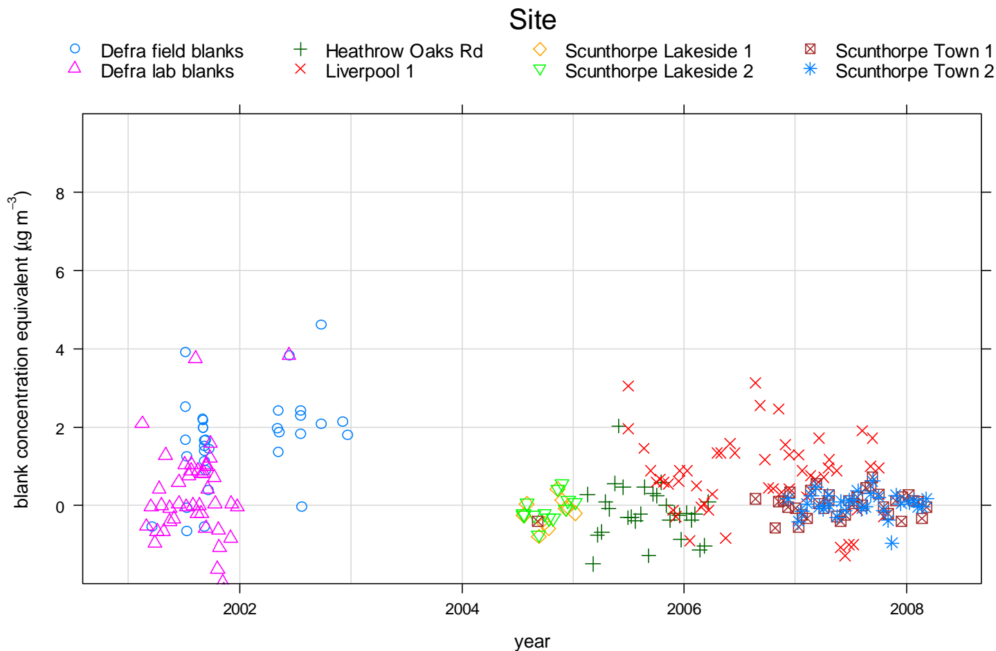
Figure 4.10 Variability of the laboratory blank concentration equivalent for Whatman QMA quartz Partisol 2025 filters weighed by AEA. Travel (field) blank concentration equivalents are also shown for the Defra research sites.
