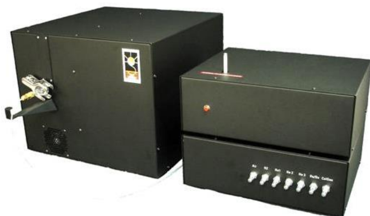
Figure 2-4 Sunset Laboratory Inc. thermal/optical carbon analyser
