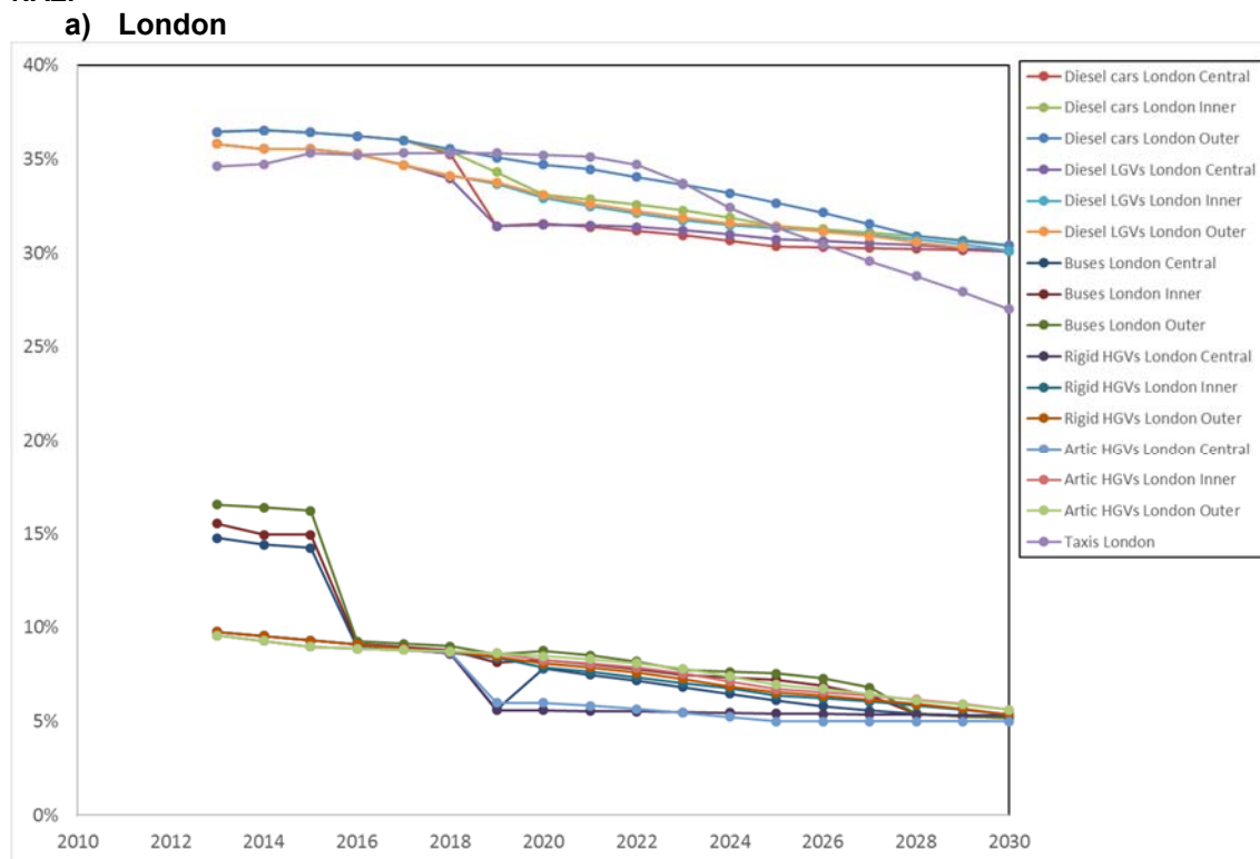
Figure 3-10 - Fleet average f\text{-NO}_2 projections by vehicle type for a) London and b) rest of the UK from NAEI
