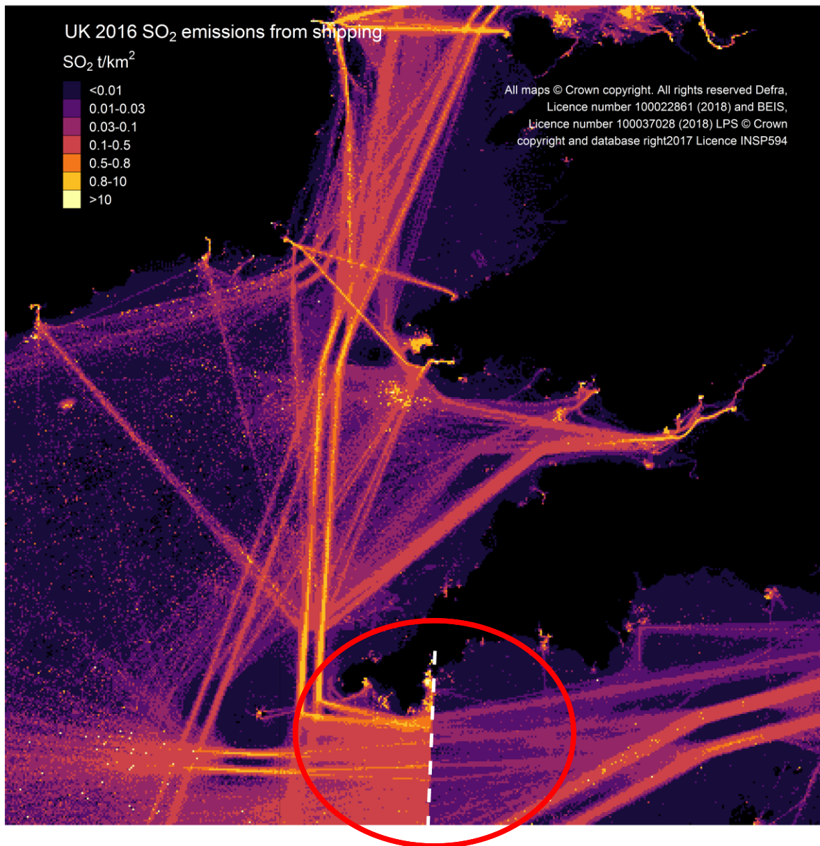
Figure 11-8 SO x emissions from all shipping around the south-west of the British Isles. The SECA (Sulphur Emission Control Area) to the east of the dotted white line (bottom centre) can be seen as a reduction in emissions
