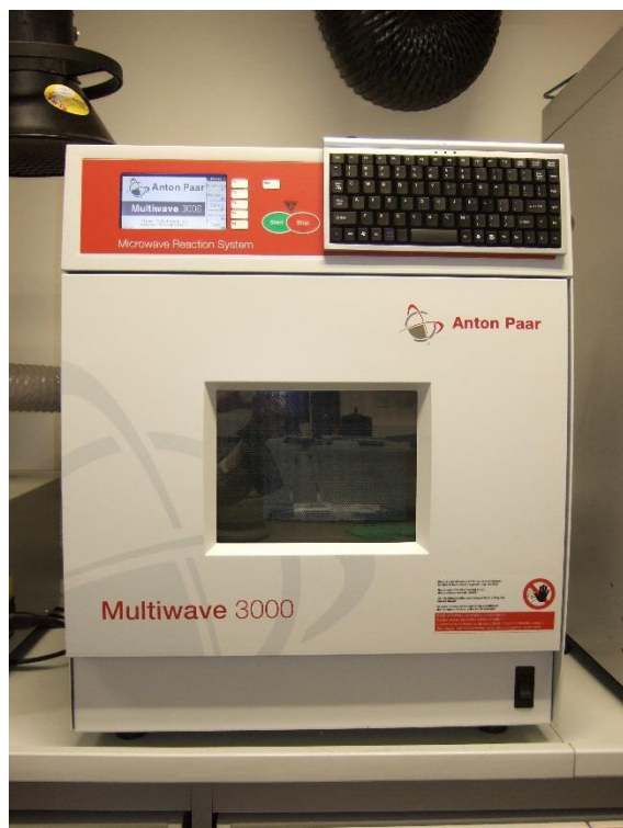
Image 2: Anton Parr Multiwave 3000 microwave used for acid digestion of the sampled filters.
