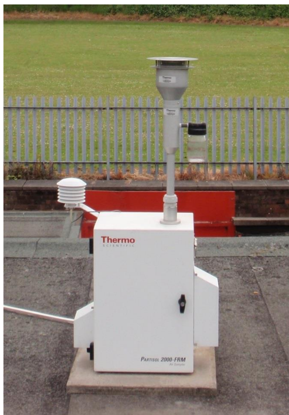
Image 1. The Partisol 2000 sampler at the Network monitoring site at Runcorn Weston Point. The inlet for the mercury vapour sampling equipment is located on the bottom left, below the white hood.
