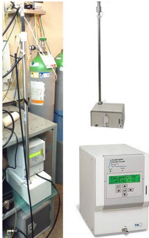
Figure 2 - CPC and drying unit equipment at a typical site
