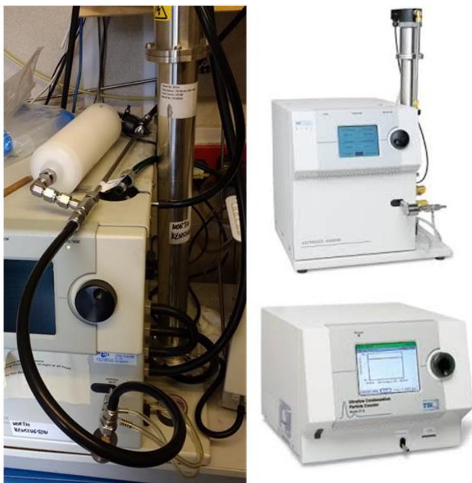
Figure 3 - SMPS and NPL drying unit equipment at a typical site
