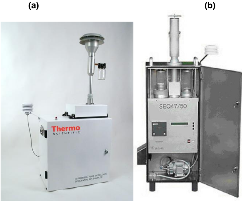
Figure 5 - (a) Thermo Partisol 2025 sampler (b) Leckel SEQ47/50 sampler
