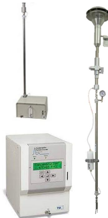
**Figure 2 - TSI 3772200 drying unit and TSI 3772-CEN-7 CPC (left); TSI 3750200 sampling system (right), photographs courtesy of TSI Incorporated.**
