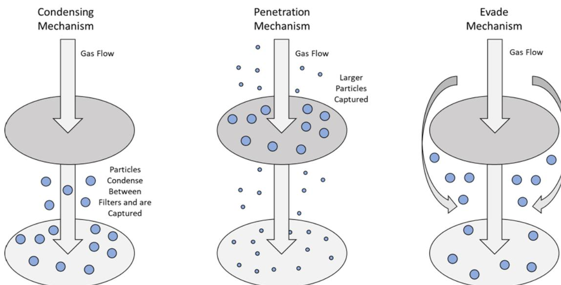
Of the three mechanisms shown in Figure A 26 the one of concern to the test programme is the evade mechanism. Due to the question posed by the filter clamping during the audit, the investigation has set out to quantify this mechanism.
