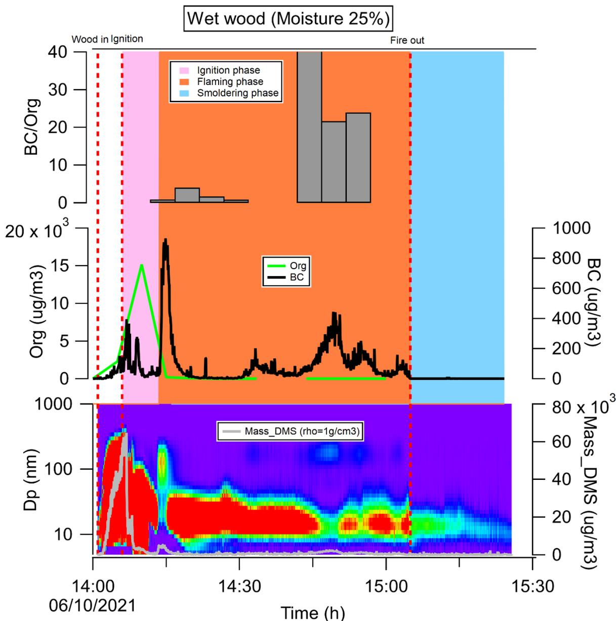
The preliminary results were used to inform the appropriate collection of samples for EC/OC analysis and to verify that the PM<sub>2.5</sub> collection strategy for the Dekati sampler was appropriate, as well as for the determination of flaming and smoldering zones.
