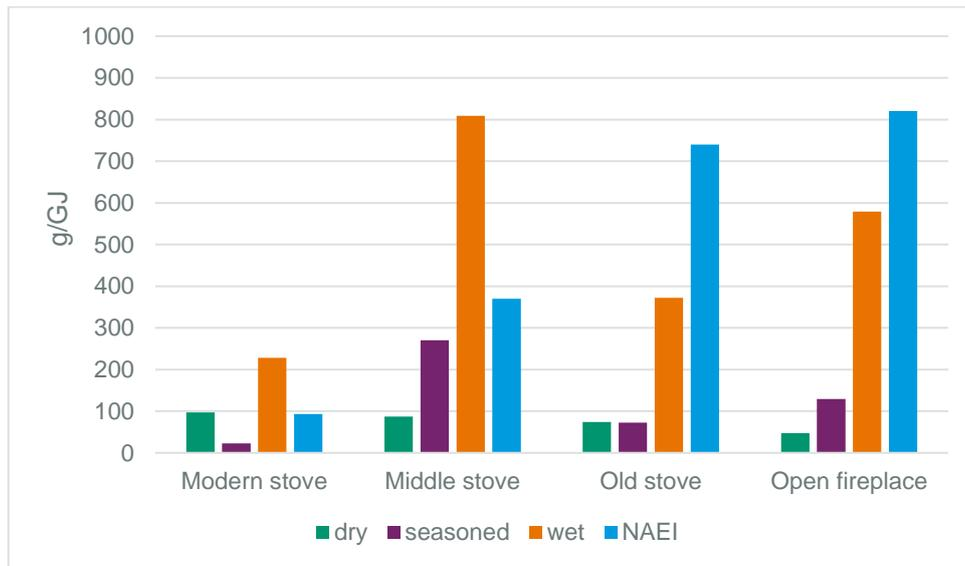
Figure 7-5 provides the condensable PM emission factors determined from the difference between total PM determined at the dilution tunnel (based on the particle size measurements) and the PM determined at the appliance outlet. Note that the NAEI reports total (filterable+condensable) PM for residential wood combustion and hence these emission factors are not proposed for use in the NAEI. The condensable PM emission factors are highest when burning wet wood for all types of appliance.
