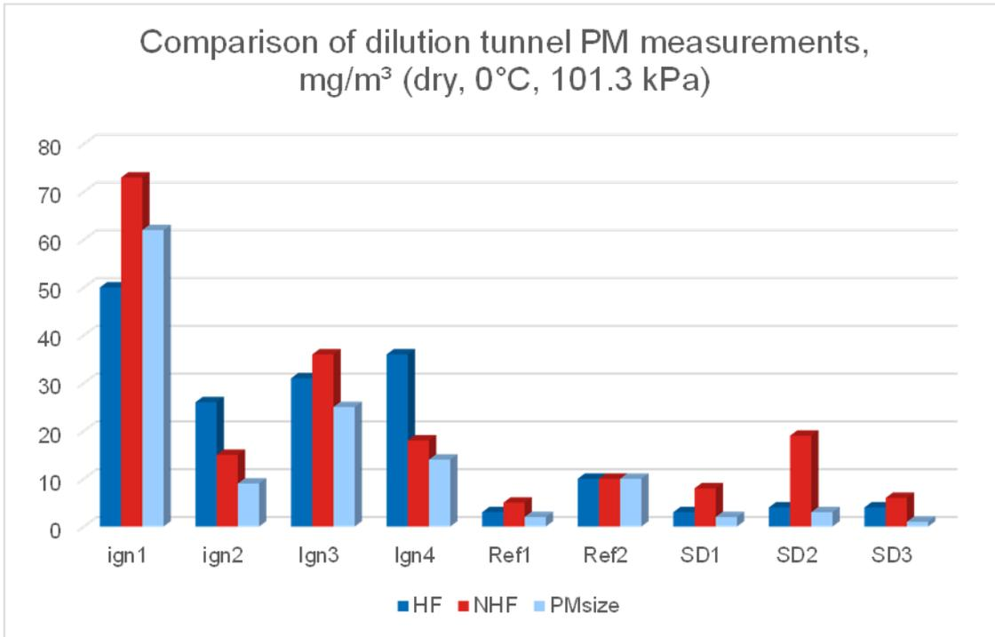
Figure A 30 : Comparison of ratio of PM concentrations at dilution tunnel to heated filter results (anthracite, modern stove)
