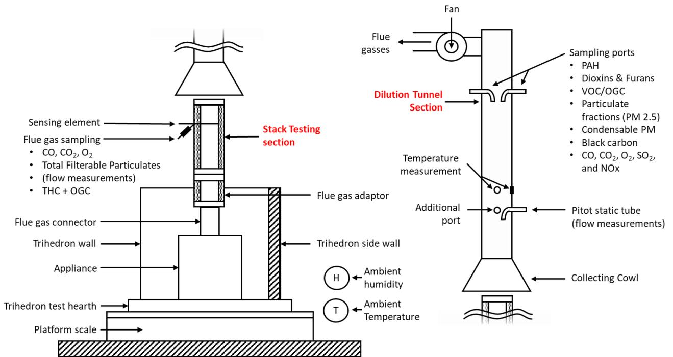
Figure 6-7: Appliance test rig
