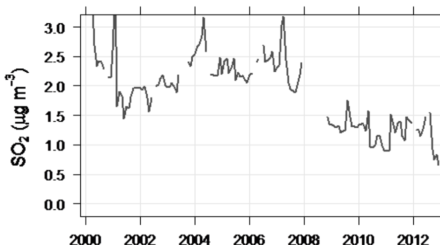
Figure 10: Time series of SO 2 concentrations at Lullington Heath for wind directions from 80° to 250°, removing the effect of long-term changes in meteorology.
