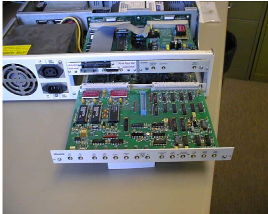
Figure (5) A photograph of the custom-made control board
