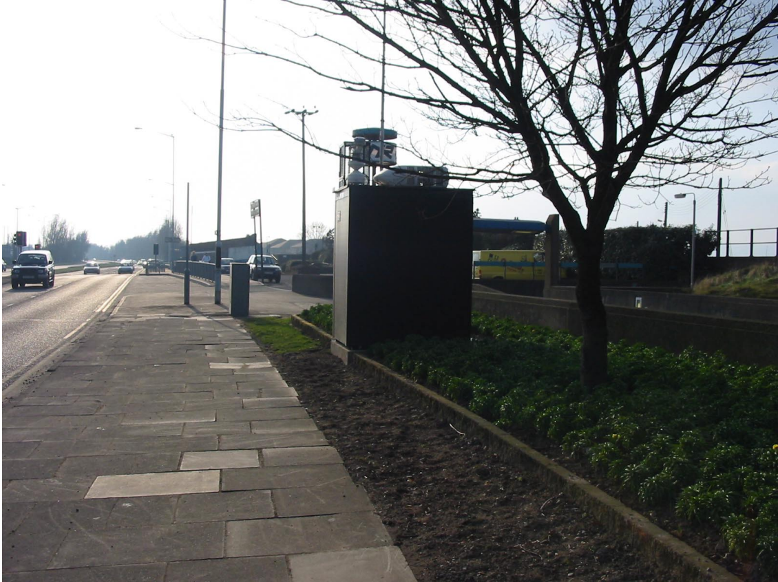
Figure 6.2 New Roadside Monitoring Site at Hollywood, North Down for PM 10 (and NO x )
