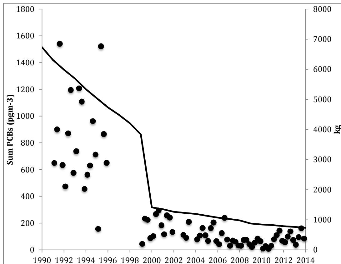
Figure 6. \Sigma_7 PCB Long-term PCB trend data from the TOMPs network for the urban (London and Manchester) and the rural (Hazelrigg, High Muffles, Auchencorth and Weybourne) sites. Data are presented as averages in \text{pg m}^{-3} and compared to the current NAEI estimates in kg per annum
