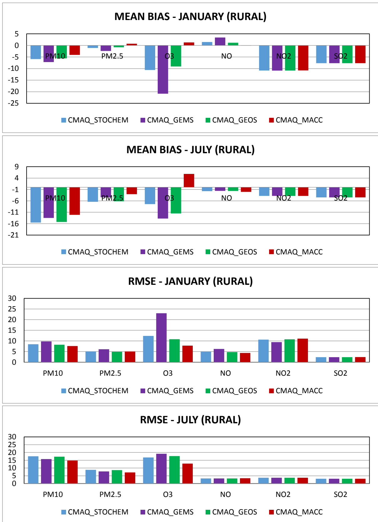
Figure 11: Mean bias and Root Mean Square Error (RMSE) of PM 10 , PM 2.5 , O 3 , NO, NO 2 , and SO 2 from different CMAQ simulations compared with the observations from rural background stations in the UK during January and July 2005
